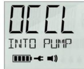
If the display shows OCCL INTO PUMP and an audio alarm sounds, the feed cannot be delivered due to a blockage between the feed container and the pump
