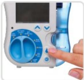
Press and hold the Prime button for 2 seconds, then release
