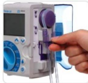
Loop pump insert around wheel, stretching lightly
